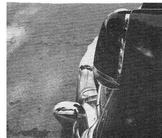
Massive chromed bumpers hug the Hudson Hornet body closely and eliminate the traditional location of the gravel pan
