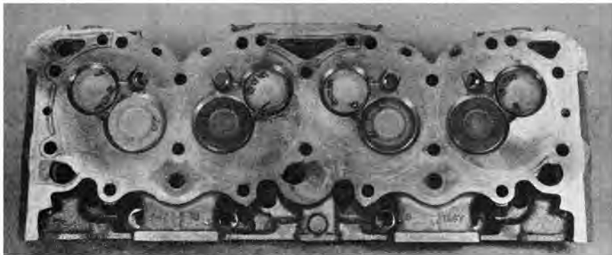
409's cylinder head has same number of valves as 348's, certainly ample. Larger bores, redesigned pistons, have un-pocketed valves.
