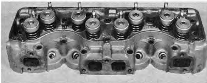
Larger valve springs with 130-pound pressure and a flat-wound spring damper are used in combination with different retainers, oil shields.
