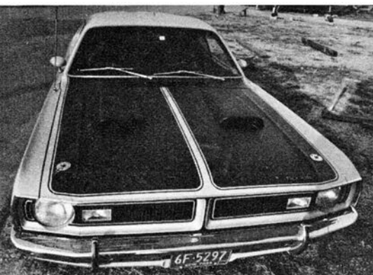
Twin scoop hood has air intake holes, but they don't mate to the carb and air cleaner.
