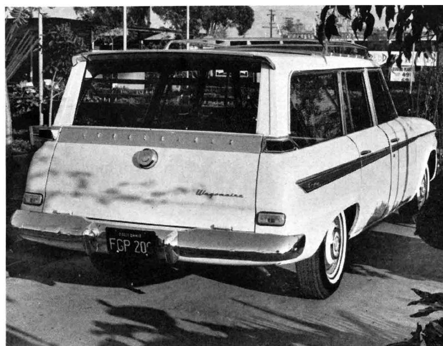
ELECTRIC REAR window operates with key twist in tailgate lock.
