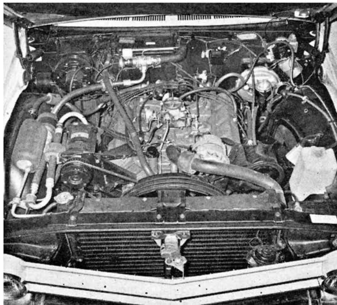
TWO-BARREL carburetor on standard version of 425-cu. in. engine chokes off horsepower, gives reasonable mileage.
