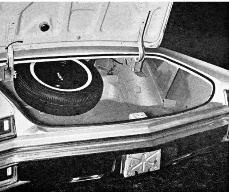
CAVERNOUS TRUNK has huge capacity, but spare location requires tire-changer to get into trunk to get out jack.
