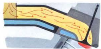
3. NEW WATER-FLOW INTAKE MANIFOLD
