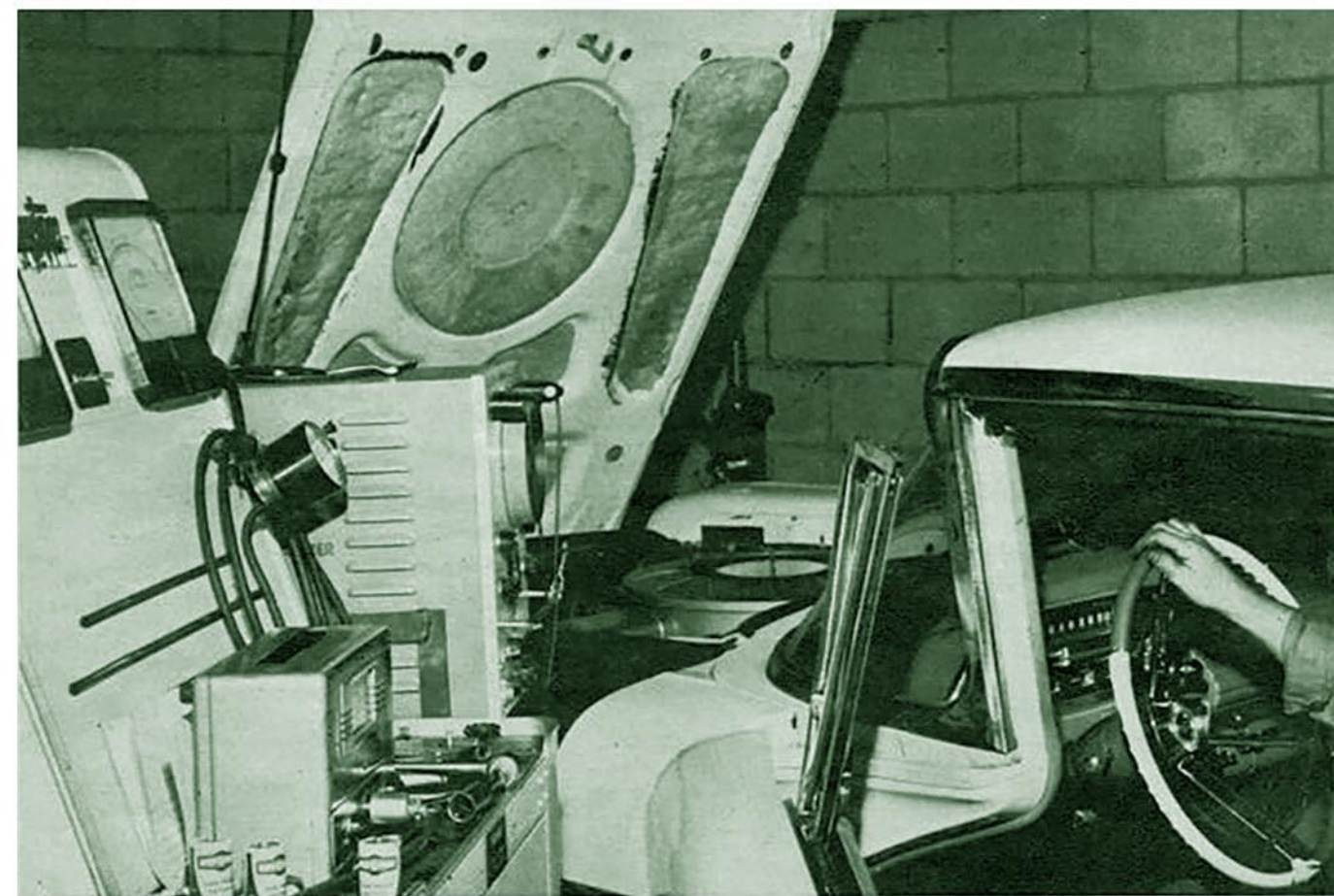
DYNAMOMETER TESTS gave 173 maximum horsepower at full load in second gear for Park Lane, 162 for Monterey engine.
