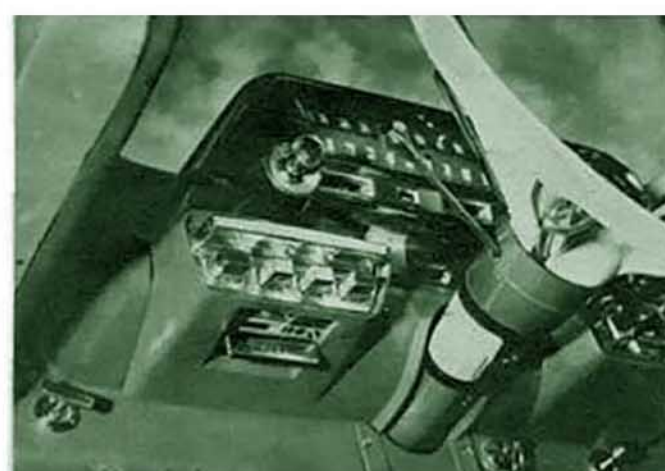
PUSHBUTTON CONTROL PANEL for gearbox hides transmission locking lever immediately below. Subdash position can mean extra blind fumbling.
