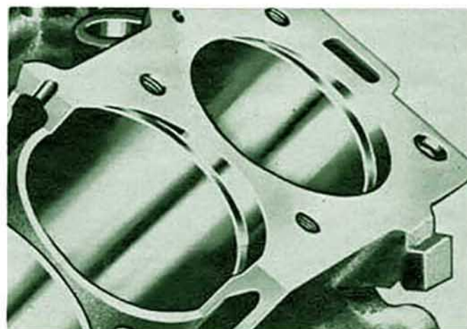
BIG 430-CUBIC-INCH ENGINE has fully-polished combustion chamber in block; top of cylinder block is machined at an angle of 10 degrees with the cylinders.
