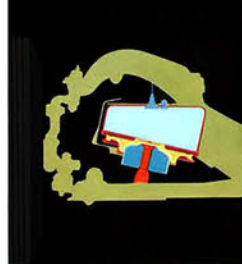
Four air springs, one at each wheel, form the basis of Oldsmobile's New-Matic Ride. This cross-section view shows the air chamber design in light blue. The piston, shown in dark blue, is in normal position, as on a smooth road. The car wheel at this point is on level ground.
