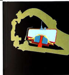
As the car wheel rises over a bump in the road, the piston is pushed up. The diaphragm expands, giving the compressed air more surface on which to press . . . and, therefore, more total resistance to the bump. Thus, despite the wheel's position, the body rides smooth and level.
