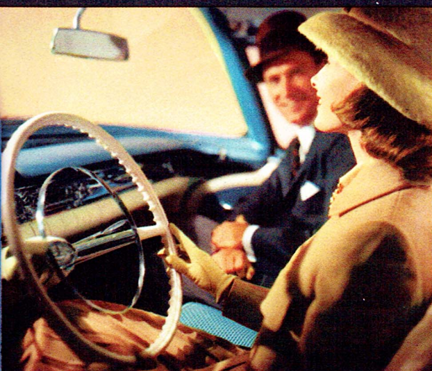
Safety Power Steering takes over 80% of the work in the '57 Oldsmobile . . . lets you drive and park with new ease and safety, yet retains the true "feel of the wheel." When the engine is not in operation, a simple bypass switches you to conventional steering.
