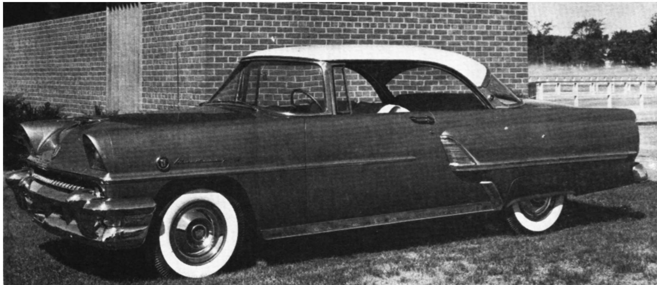
Monterey profile shows new headlight shade rake, new grille-bumper assembly, wrap-around windshield and higher rear fender treatment.
