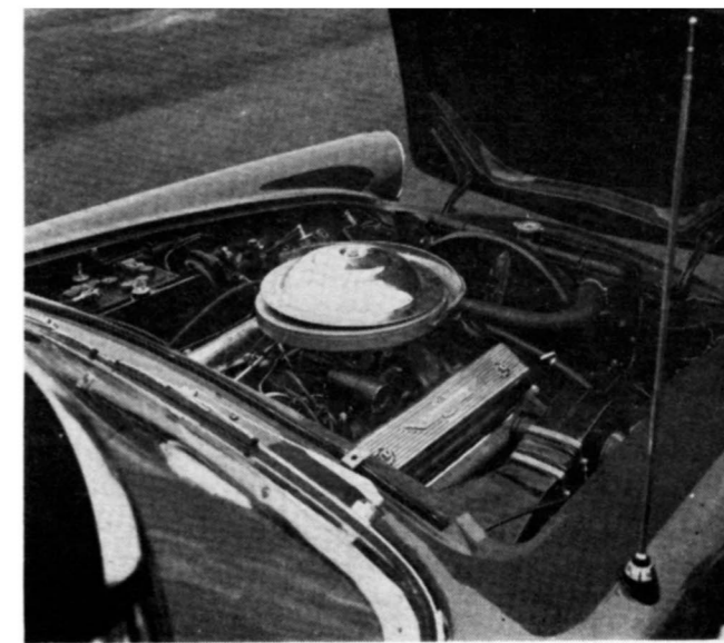
Power plant is 292 cubic inch ohv V-8 with single four-throat carburetor and dual exhausts. The Thunderbird exceeds 115 mph.
