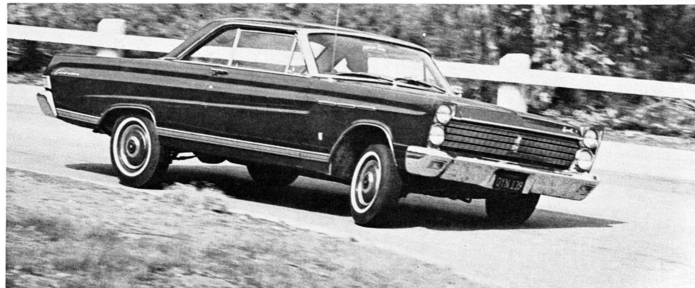
CALIENTE DIDN'T HAVE KIT AND WAS FOUR TO FIVE MPH SLOWER FOR SAME DEGREE OF CONTROL IN TURNS LIKE THIS. LEAN WAS MODERATE.
