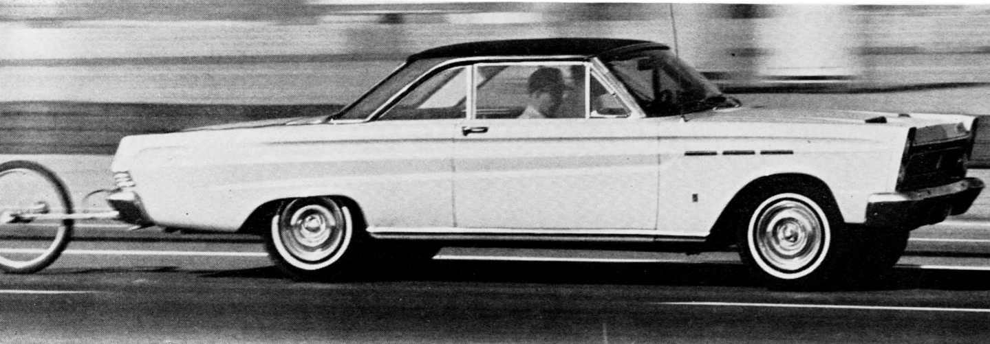
COMETS WERE STABLE AT HIGH SPEEDS. ENGINE AND DRIVE-LINE NOISES DIDN'T INCREASE APPRECIABLY, BUT WIND NOISE WAS QUITE HIGH.
