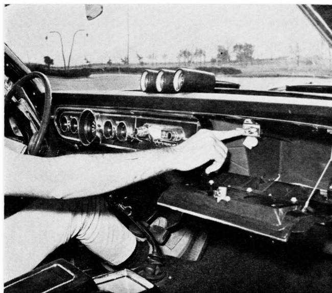
Remote trunk lid release can be reached from driver's seat. Tach, clock, and vacuum gauge atop dash are small but readable.
