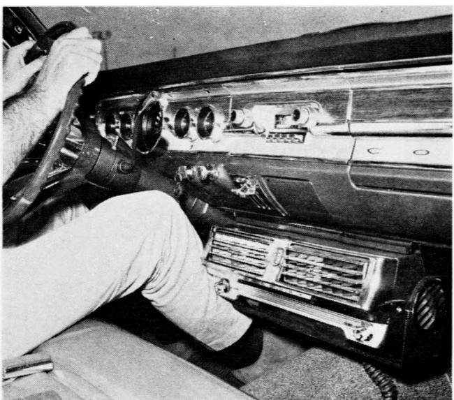
Caliente's air conditioner interfered with driver's right leg. Relocation toward passenger side would be a great improvement.
