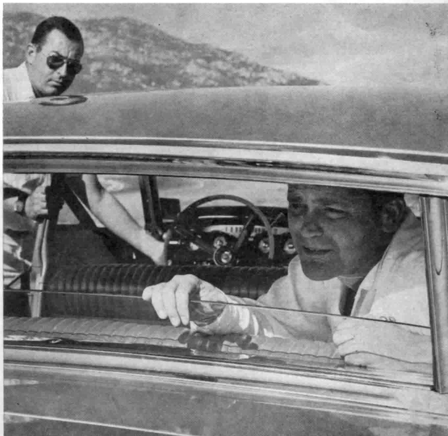
REVERSE-SLANT REAR WINDOW WAS FIRST INTRODUCED BY LINCOLN A FEW YEARS BACK. DASH CONTROL ALLOWS IT TO BE RAISED, LOWERED.
