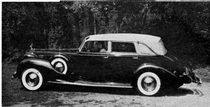
MAJESTIC 1938 Packard Twelve was forerunner of later cars with tinted glass. Coachbuilder Brunn inserted a dark green glass panel above each high, narrow half of V windshield. Car was called a cabriolet because of fabric top with convertible rear quarter. Interior hardware was silver over bronze; cushions were stuffed with eiderdown. Three-ton monster cost $9600 new, was basically a stock V-12 of 175 horsepower, 139-inch wheelbase, 220-inch overall length, 473-cubic-inch displacement. Lucky owner: Albert E. G. Sellers, Radnor, Pa.
