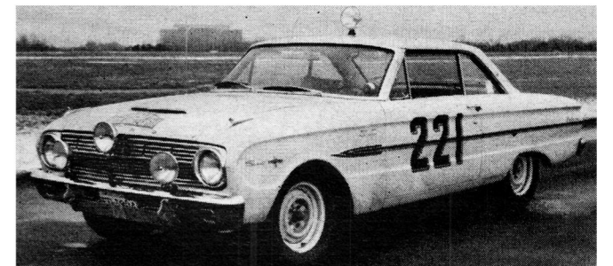
This is serious business, men. All auxiliary road lamps are Lucas, headlights Cibibi. The 15-inch wheels are optional Ford.
