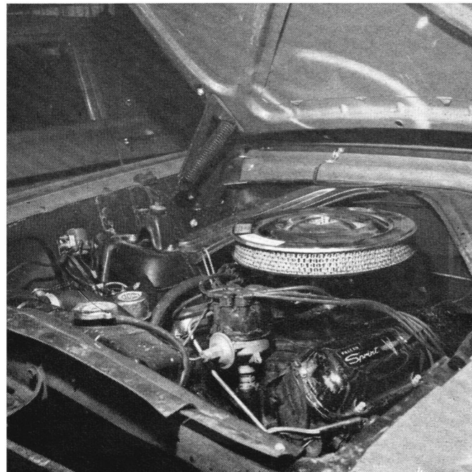
Standard Sprint's engine compartment is stuffed full of V-8 brute force where only a gentle little six was meant to live.
