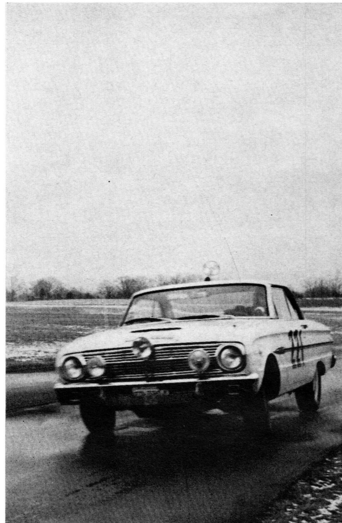
Less roll and more stability; notice acute angle of inside front wheel. Front end had 1° negative camber, 3/8-inch toe-out.
