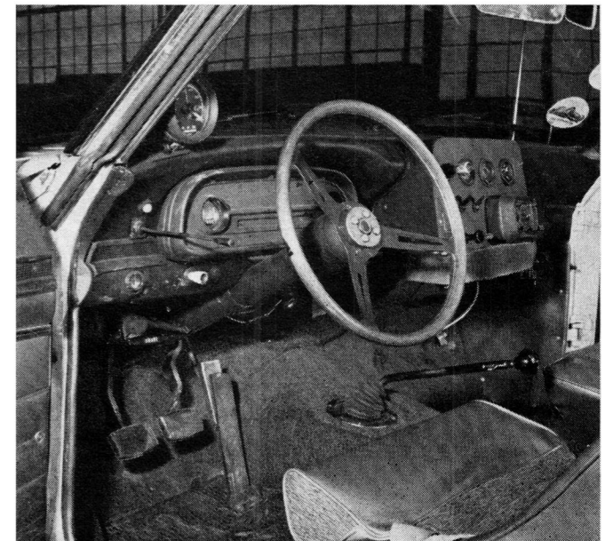
Not what you'd call jazzy, the rally car's interior is all business. Note tachometer's tell-tale lodged at 7,000 rpm.
