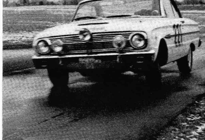
Less roll and more stability; notice acute angle of inside front wheel. Front end had 1° negative camber, 3/8-inch toe-out.
