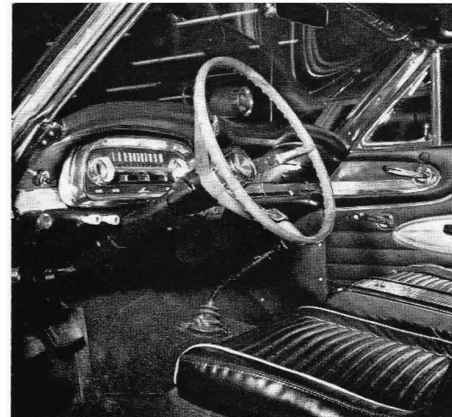
Deep-dish steering wheel intrudes upon living space, makes it uncomfortable for tall man to drive. Flat wheel would help.
