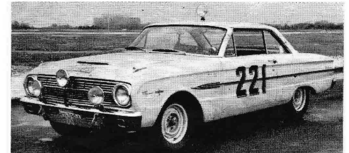
This is serious business, men. All auxiliary road lamps are Lucas, headlights Cibí. The 15-inch wheels are optional Ford.
