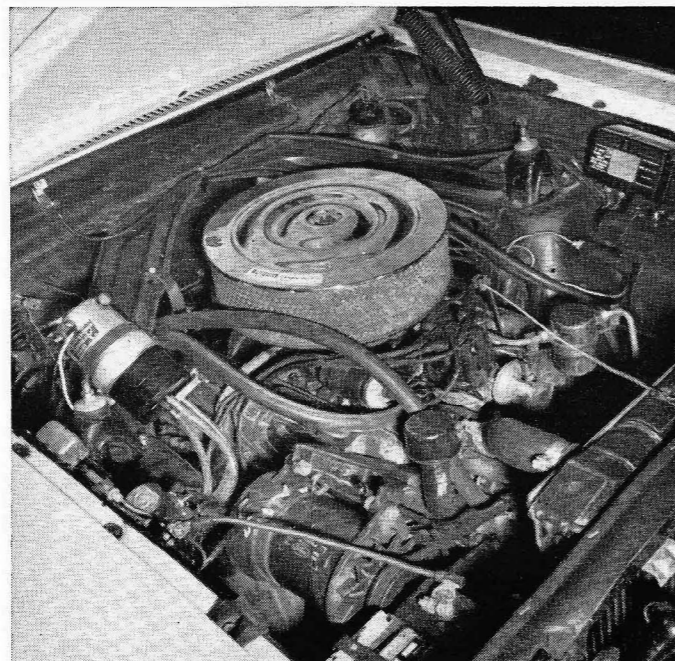
Rally Sprint's engine room shows few differences except for bigger carb air cleaner and tank for air horn (at far left).
