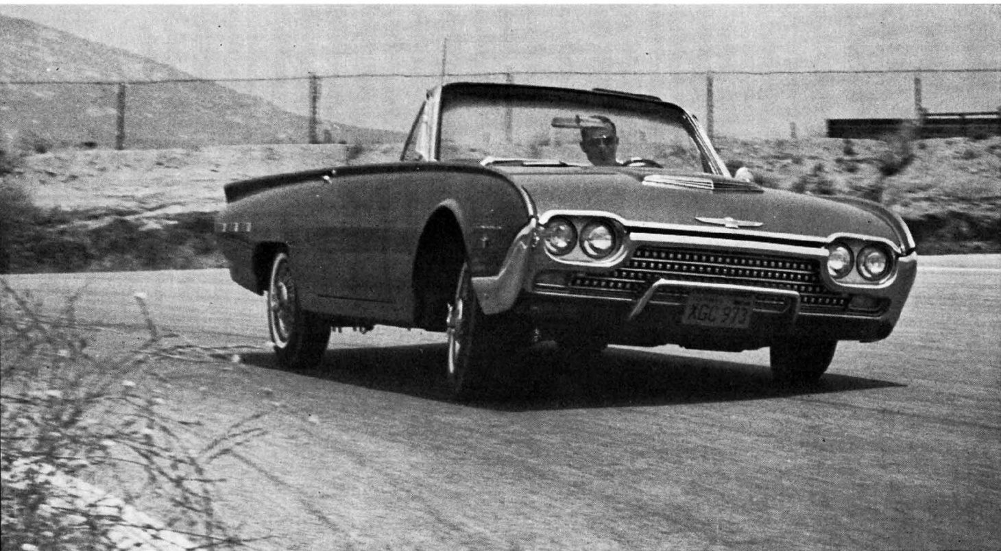
TIGHT CORNERS BRING OUT THE WORST IN THE 'BIRD, AS UNDERSTEER AND BODY ROLL ARE EXCESSIVE AND DETRACT FROM OVERALL COMFORT.
