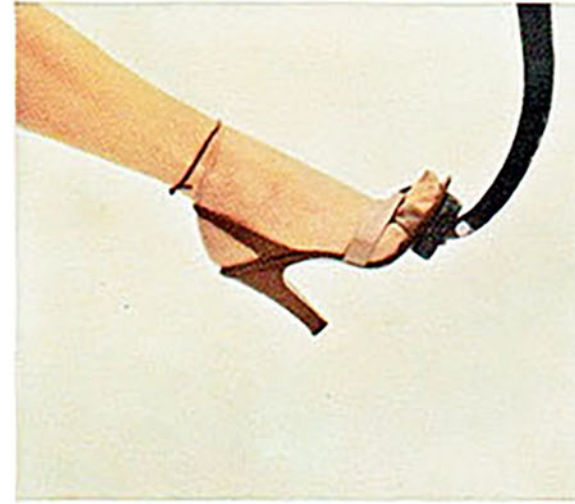
Lincoln's power brakes require up to 50% less foot pressure. Design of the suspended brake pedal lets you pivot from accelerator to brake without having to lift your foot.
