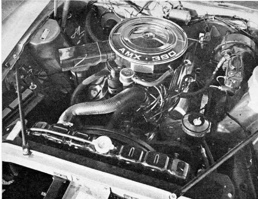
NEW ENGINE is same basic block as 290 and 343-cid engines, occupies same volume, but has extensive internal reinforcement for improved life.
