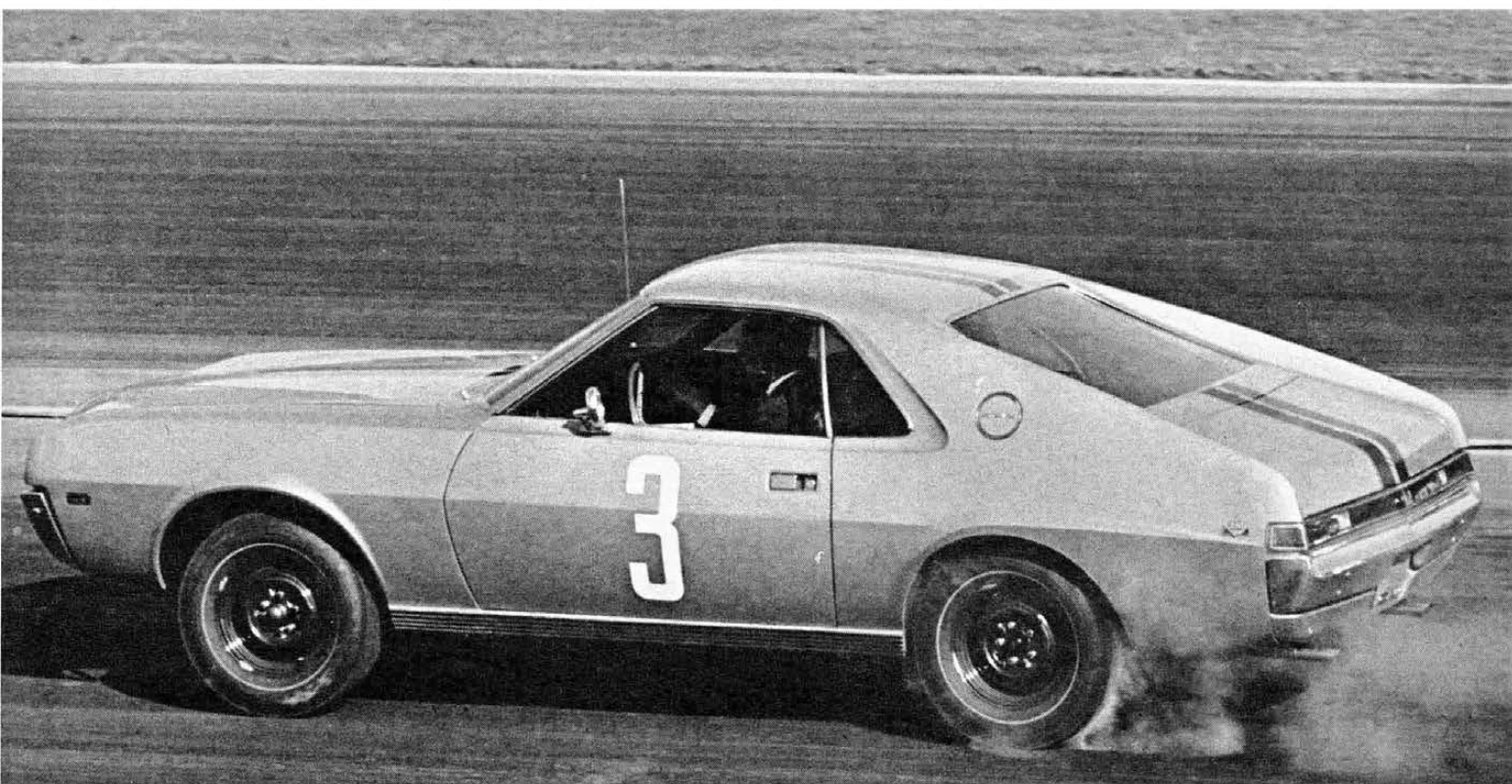
TOP ENGINE option provides far more torque than can be transferred to pavement by standard tires. Engine is tuned for torque, rather than high-end horsepower, a rather poor compromise for lightweight AMX.
