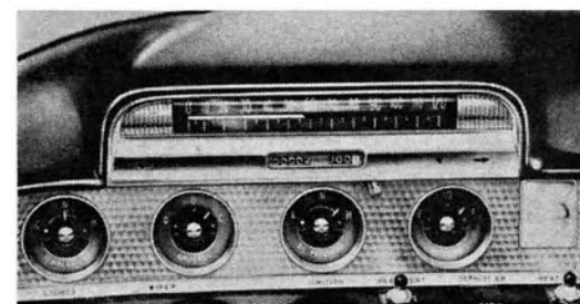
Secret of "Redliner" speedometer is red-and-black drum (above), which turns up red line across panel, eliminating needle. Buick's instrument panel (right, above), modeled after "Wildcat" panel, is double-roll type, with all instruments in front of driver for maximum readability. "Redliner" speedometer is shown in detail at right
