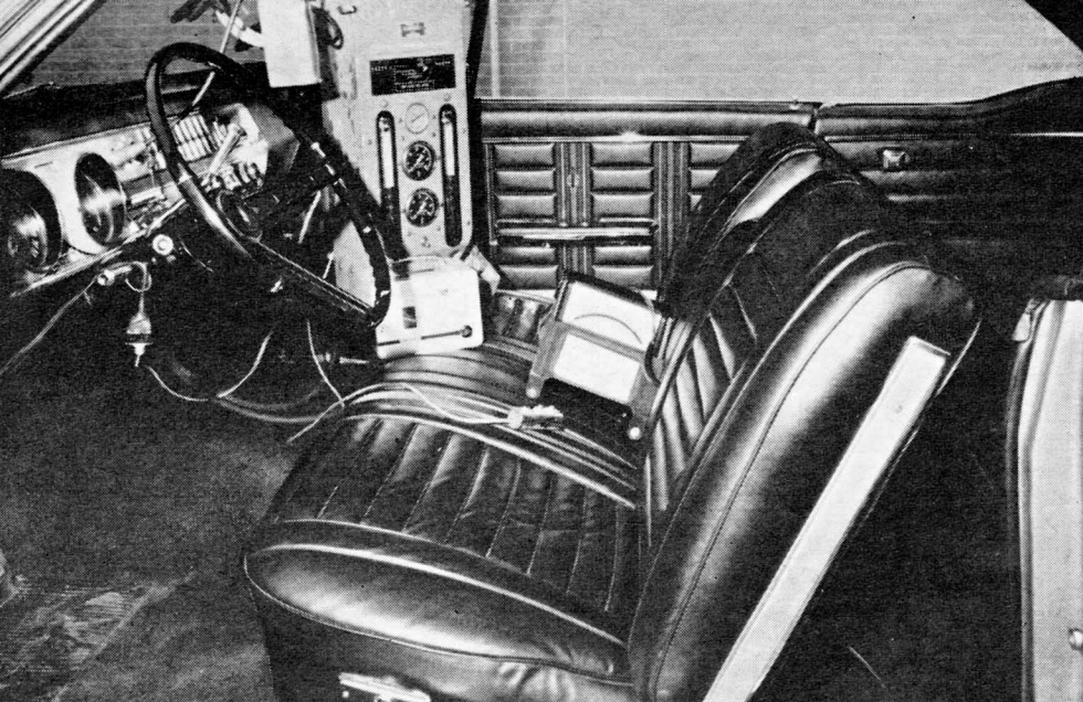
FUEL FLOW meter, electric tachometer and decelerometer were used to test the Oldsmobile Turnpike Cruiser's performance on GM proving ground.
