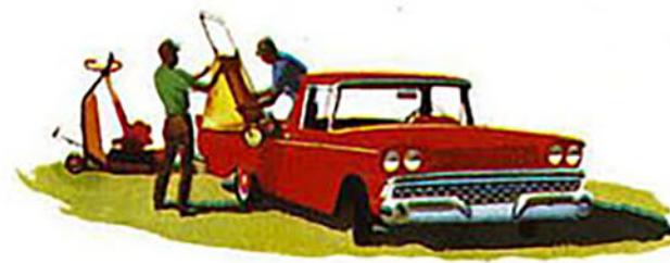
EXTRA STRENGTH —Ranchero has the heft to handle husky hauls in handy fashion. Sides, floor and tailgate have rugged double-wall construction for greater strength and rigidity.
