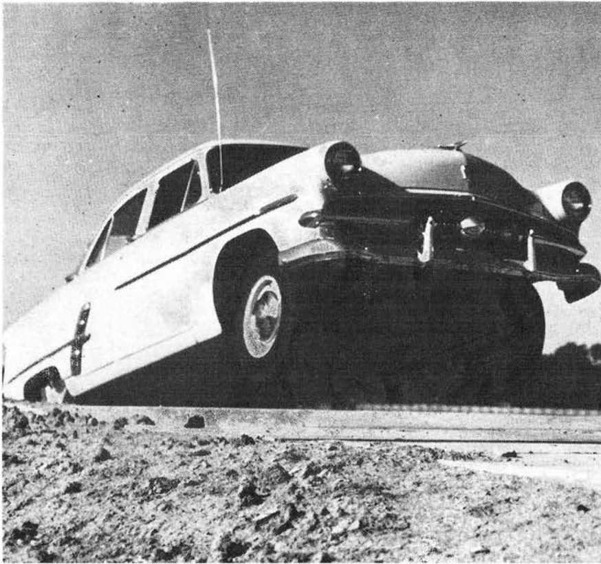
Rough treatment received by cars at Ford's track is illustrated as a '53 model powered by new ohv V-8 takes railroad crossing setup with a high bounce. Tests like this also gave new front end suspension system a severe beating and demonstrated the easier handling characteristics as well as simpler repair operation
