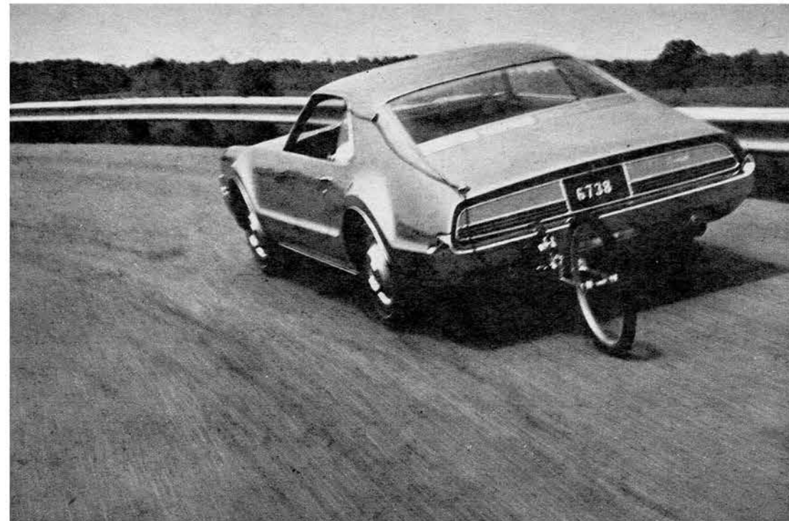
Even a fifth wheel has its function! This one is calibrated to fractions of a mile-per-hour. Records every move the Toronado made in miles and miles of grueling performance around the Proving Ground track. Supplies data for evaluating the test car's response under varying performance conditions.
