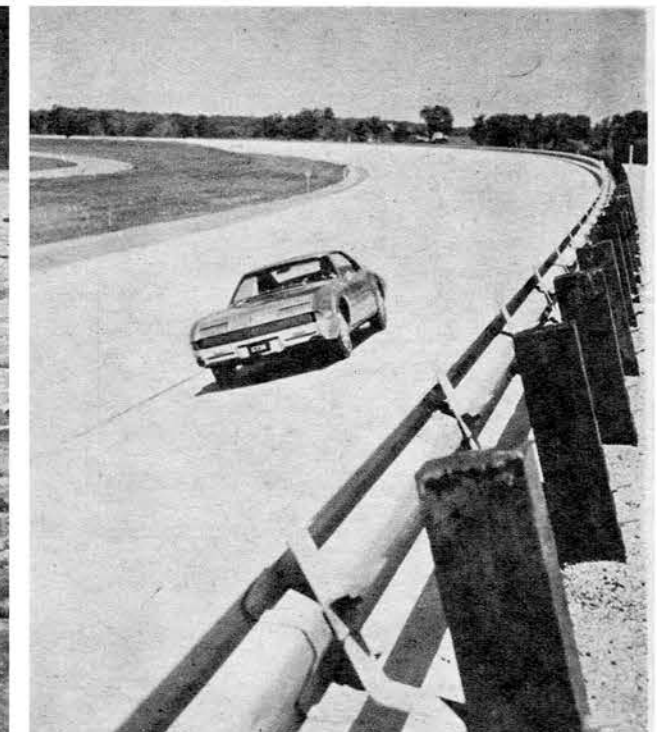
Round and round she goes! Mile after mile on the high speed oval measures Toronado's durability. Stops are made only for fuel and routine maintenance.
