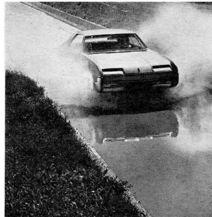
Thorough dunking! Toronado passes water trough test with flying colors! Electrical system gets the acid test. Salt water checks out corrosion resistance of critical components.
