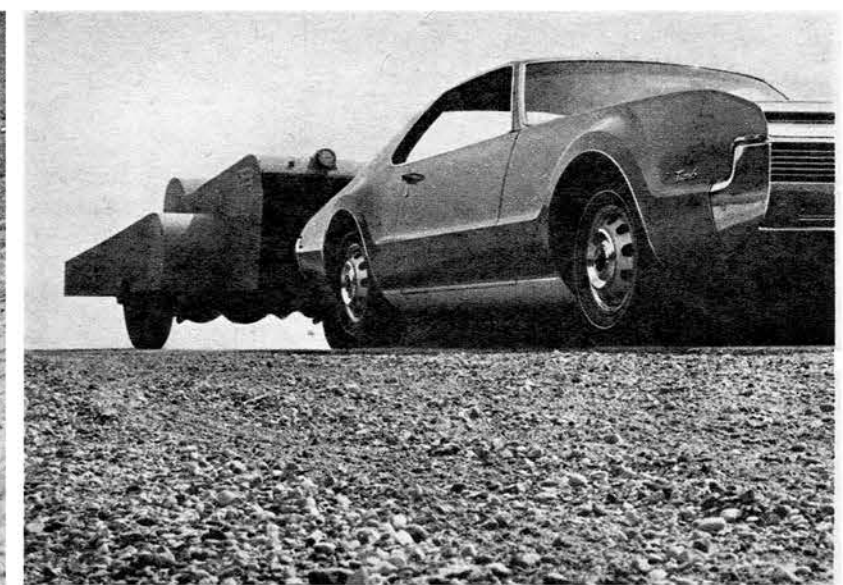
Two-ton tow! Four-thousand-pound dynamometers are towed hour on hour, simulating various grades and driving conditions to produce accurate readings on the road power developed by the 385-hp Toronado Rocket V-8.
