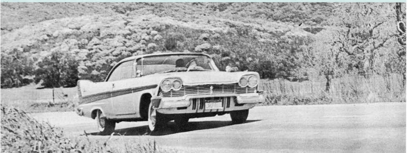
Sharp inward turn of front wheels indicates strong understeer characteristics. At cornering speeds of 55 mph, the rear wheels would slide outward very gradually. Body roll was very slight.
