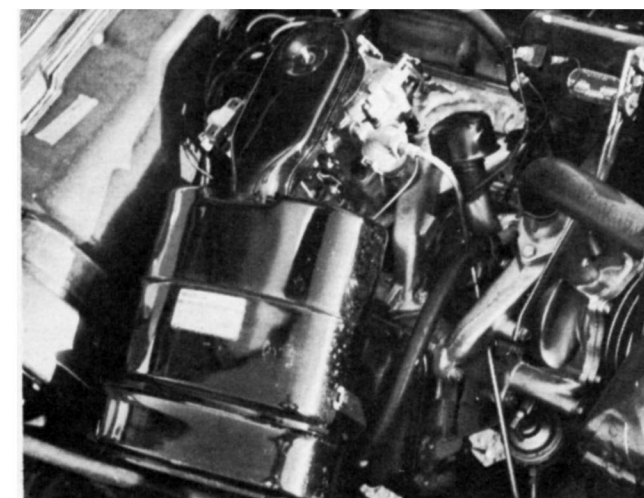
Like many '57's, Dodge uses paper air cleaner for easy service and low hood. Element is blown out at 6000 miles and thrown away at 12,000. Other access good.
