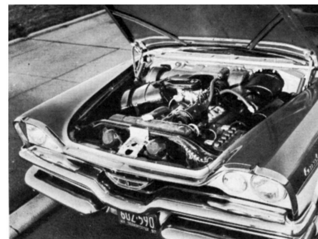
Counterbalanced hood opens wide, reveals fully-packed engine room. Heater and blower bulkhead-mounted in fiber case, left of bellows for brake servo.
