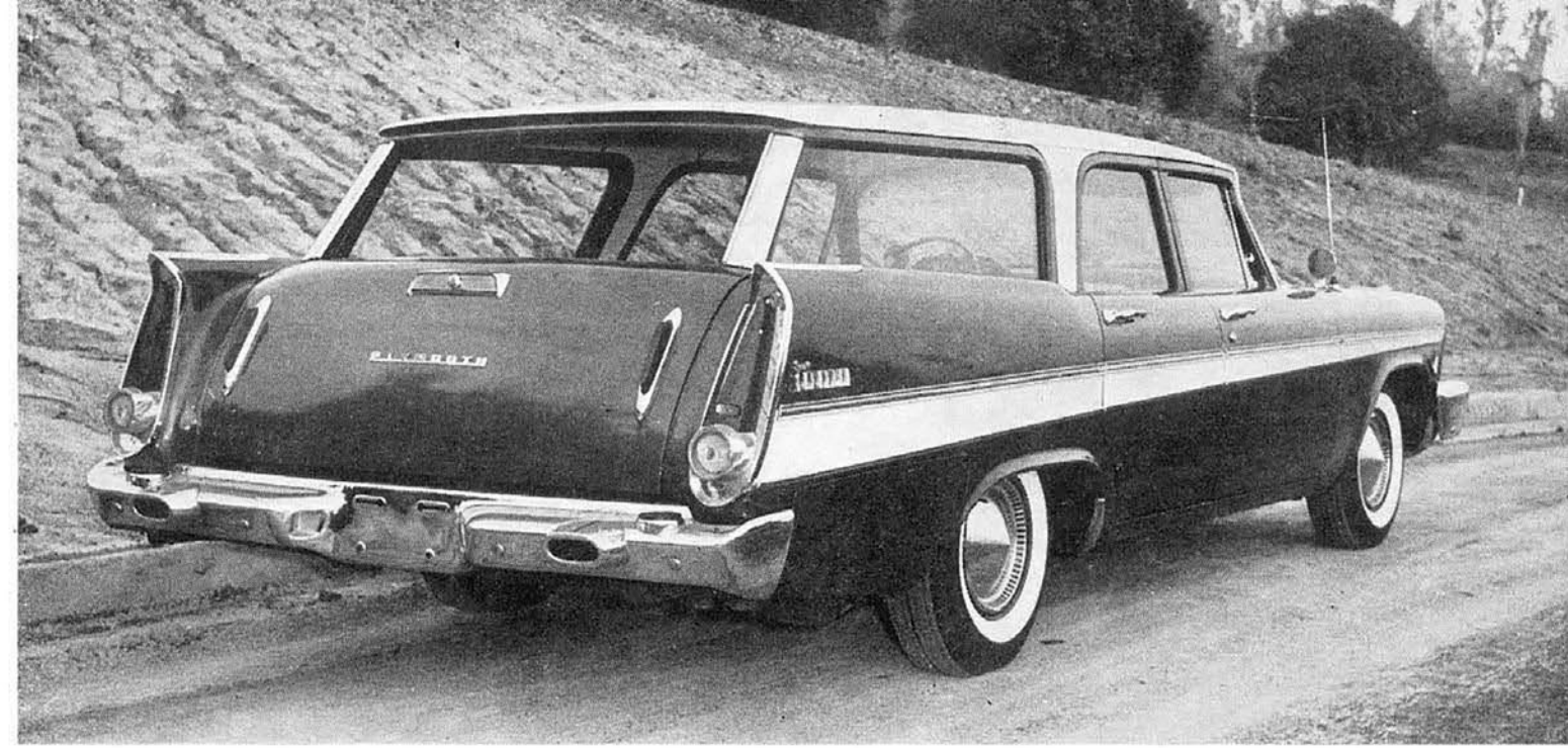
AMONG THE RADICALLY NEW FEATURES IS THE SPARE TIRE CLEVERLY CONCEALED INSIDE AND LOWERED FROM THE RIGHT REAR FENDER.
