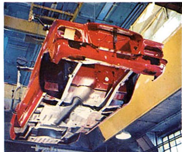
This is the one-piece solid body-frame from Chrysler Corporation, welded into an integral, girder-like, fortress that practically eliminates every kind of squeak, rattle or groan.
