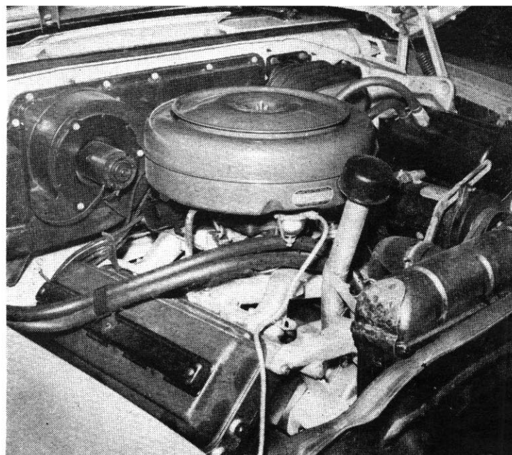
Back to the hemisphere for the 315 cu. in. D-500 engines. Old style rocker covers are the clue. Engine is easily accessible.
