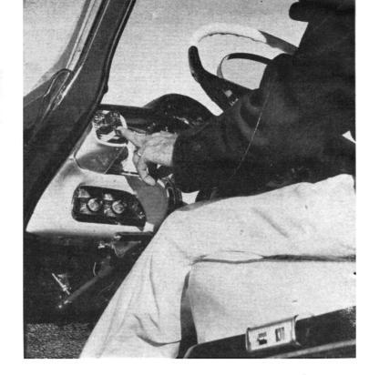
PUSHBUTTONS are the ultimate and logical system of automatic transmission control. Dodge's buttons—neutral, drive. low. reverse—seem handier at the left than the former righthand gear lever. need but a flick of a finger to operate. Driving with them took no big adjustment in habits. and the new ease is as much mental as physical. Operation actually is more precise than with the conventional quadrant.
