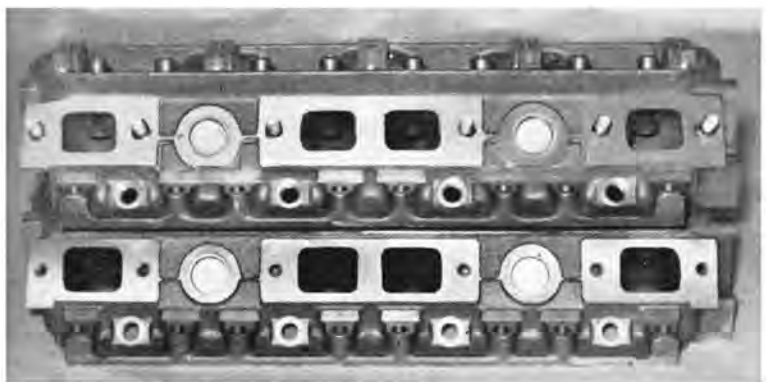
LEFT—Exhaust ports on the new cylinder head, bottom, are 25% larger than standard 413 head. These larger ports, larger exhaust valves and large capacity exhaust headers should be an important improvement in the new engine. RIGHT—Seen from the intake side, new cylinder head, bottom, does not have heat crossover passage, the intake ports are visibly much larger. With new short ram intake manifold, this combination should be the best in the industry.
