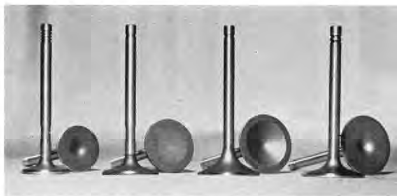
LEFT—Valve train for the new engine has been proven stable at 6500 rpm, consists of: Flat side lifter with extra clearance, tubular pushrod, cast adjustable rocker arm, steel retainer washer with single bead locks, dual springs and new valves. RIGHT—From left: Standard 413 exhaust, H-D exhaust, H-D intake, standard 413 intake. New H-D exhaust is \frac{1}{4} -inch larger and has better contour under head. H-D intake is same size but has much deeper tulip and improved flow contouring.
