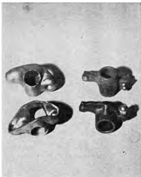
LEFT — New pushrods, center, are \frac{3}{8} -inch tube with .083 wall and tip inserts. Standard pushrods are solid \frac{5}{16} -inch. CENTER — Standard 413 rockers, left, are stamped steel. New H-D versions are cast, have adjusting screw and locknut. RIGHT — This is the factory installed exhaust system that will be fitted to Dodge and Plymouths with 410, 420 hp engines.
