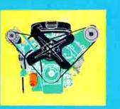
This full-size, 394 cubic-inch Rocket Engine . . . developing a lively 250 horsepower . . . is standard on every Dynamic 88. Econ-O-Way Carburetor and minimum overlap camshaft precisely monitor fuel flow to assure maximum mileage. Special dished pistons allow a compression ratio of 8.75-to-1 for Rocket "Go" on regular gas. Skyrocket Engine is optional at extra cost on Dynamic 88s.
