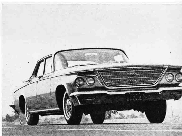
Although not a neck-snapper, Newport got off line smartly, nearly matched more powerful New Yorker's acceleration despite rather tall gearing designed for long-range cruising economy.
