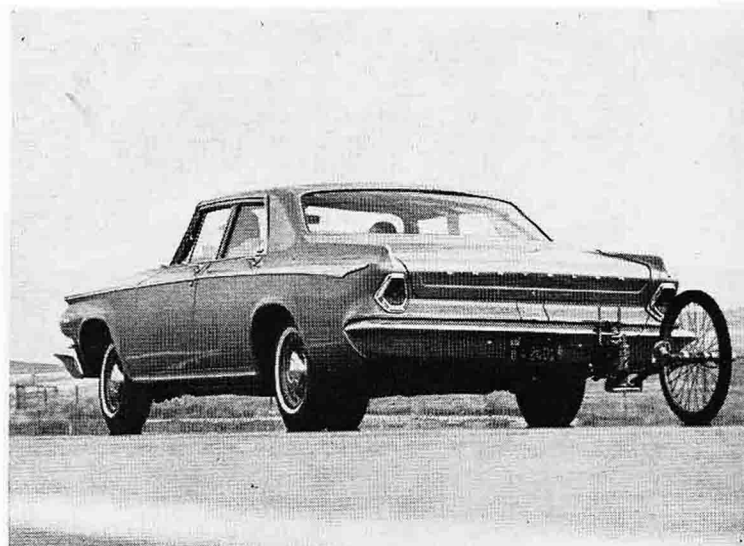
Newly designed tail lights and revamped rear deck distinguish test car from 1963 models. Even under maximum acceleration, Newport showed little rear-end squat or spinning of wheels.
