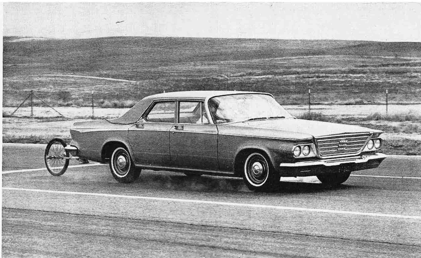
HUSKY 11-INCH-DRUM BRAKES, WITH BONDED, EXTRUDED ASBESTOS LININGS, GAVE POWERFUL STOPS, WITH GOOD CONTROL, LITTLE NOSE DIVE.
