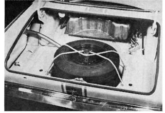
For 1964 Scott and his teammates have switched to new V8-powered Valiants in an effort to further prove model as a rally natural. Extension post for wheels permits quick spare change. Ahead is auxiliary tank, valve, emergency pump.
