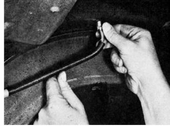
The fuel line to the auxiliary gas tank, in an exposed position, is protected with a coil wire shield. The Valiants are groomed for the Monte Carlo Rally which, like the Canadian 4000, is extremely difficult, under worst conditions; driver and navigator spend up to 22 hours a day in car on big runs.
