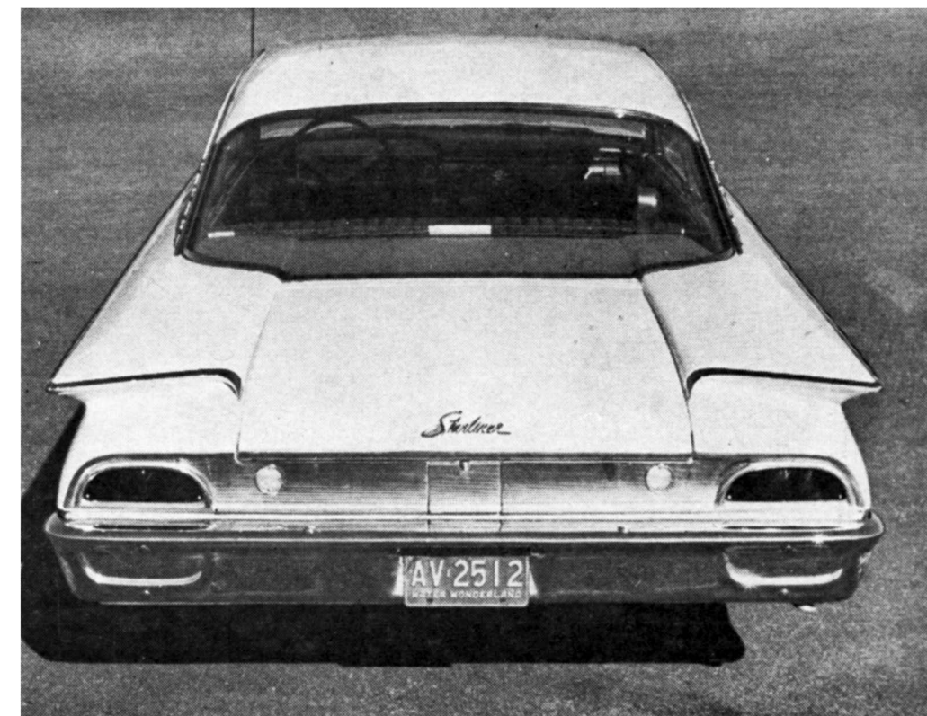
Maximum width across Ford's swept-back fins is 81.5 inches while the rear window on the hardtop Starliner has nearly 30% more area than the front wrap-around windshield.
