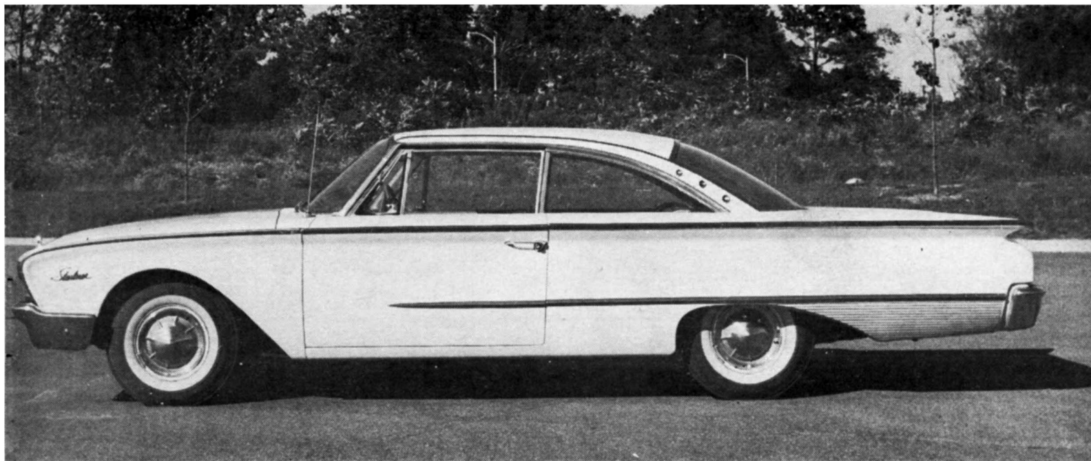
Sleek lines for 1960 Ford Starliner also contribute toward top speed. Notice that Ford now uses swept back windshield post so that passengers can enter and exit without bumping the troublesome "dogleg" corner as used on windshields in the past.
