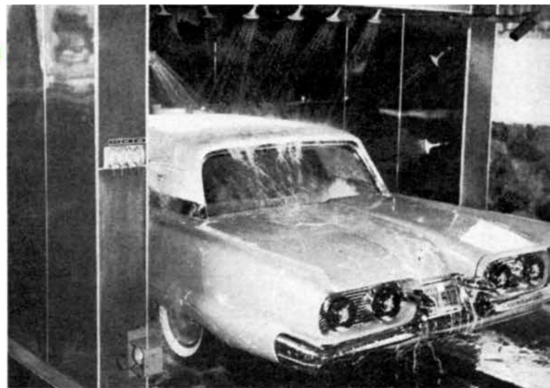
1959 T-Bird made the trip through high pressure water spray without showing signs of leakage around doors or windows. Many of the cars we test do leak badly on this same wash rack.
