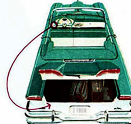
AUTOMATIC REAR DECK OPENER. —Dash-mounted key-lock switch opens compartment from driver's seat. Different key opens deck lid from outside. Optional.
