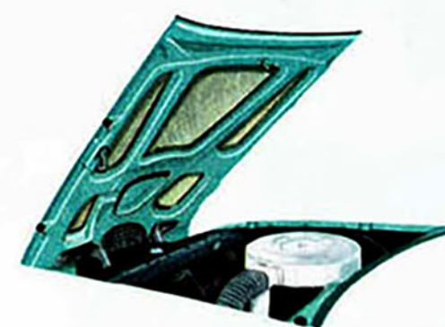
INSIDE LOCKING HOOD. —The hood of the Edsel is released from the driver's seat as an added protection against tampering with engine, battery and underhood accessories.
