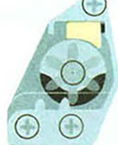
NEW SAFETY DOOR LATCHES. —Because they rotate into engagement between specially designed interlocking plates, Edsel door latches not only close easily, but also hold firm against both up-and-down and side-to-side movement.
