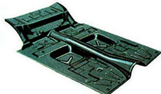
NEW ROOMINESS AND COMFORT. —Built-in footrests are stamped deeply into Edsel rear compartment floor to add valuable legroom and increase passenger comfort. The inherent rigidity of this formed steel stamping is further increased by spot-welded reinforcements.
