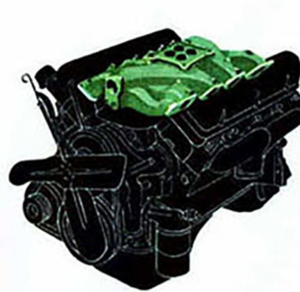
WATER-WARMED INTAKE MANIFOLD. —For quicker peak performance after starting, Citation and Corsair engines are designed with a water jacket in the intake manifold. Water from the engine cooling system is circulated through passages in the intake manifold to provide quick engine warm-up as well as more even stabilization of the fuel-air mixture for maximum performance and economy.
