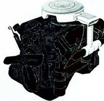
TEMPERED AIR INDUCTION SYSTEM. —On Citation and Corsair models, a unique air induction system is used. This system provides the carburetor with air at just the right temperature. In cold weather, air is exhaust-heated for quick warm-up. When the engine is warm, the system switches automatically to cool outside air. In hot weather, the cooler outside air, because it is denser, provides smoother, quieter engine operation.
