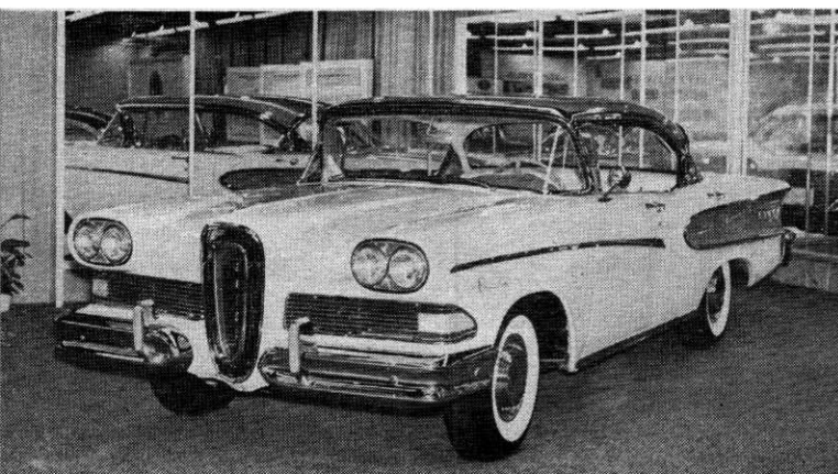
PACER SERIES is the top series in the lower half of the Edsel lineup. With the Ranger, it shares some basic Ford components. Bumper guards are mounted inboard. Grille is only radical touch.
