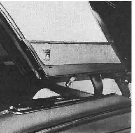
Power-operated screwdown clamps at the four corners give the "fliptop" solid, rattle-free fit.
