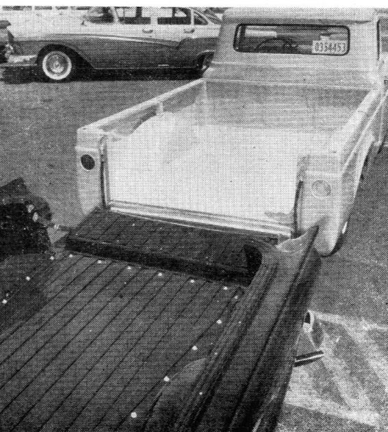
F-100 pickup bed has square rear corners and no inside paneling while Ranchero corners are rounded and interior paneled.
