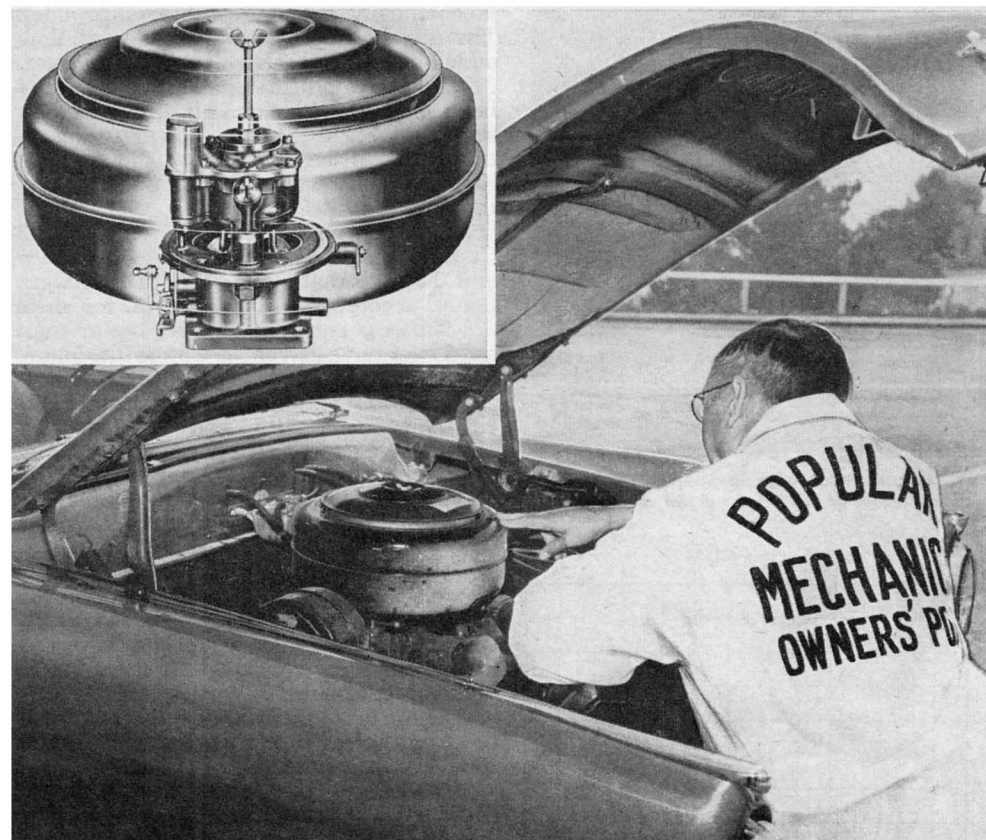
Big air cleaner surrounds carburetor instead of being mounted on top. Padding under hood deadens sounds
