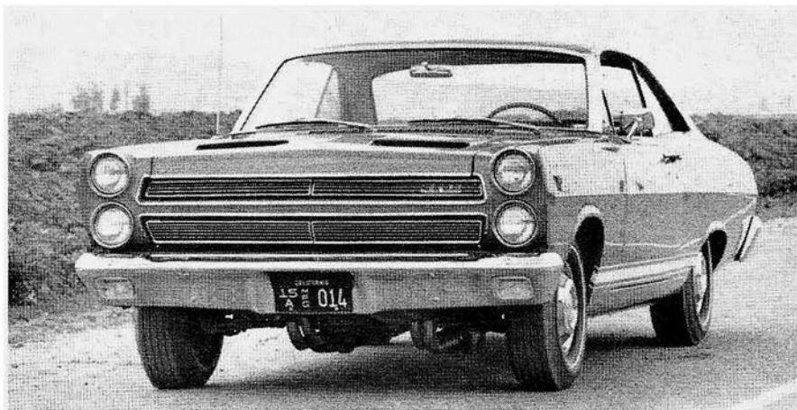
FIBERGLASS HOOD with twin air scoops heralds Cyclone GT arrival on the drag scene. Some judicious drilling would make the scoops functional.
