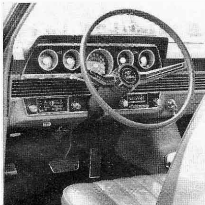
INSTRUMENT layout put everything in front of driver, but lacked a tachometer.
