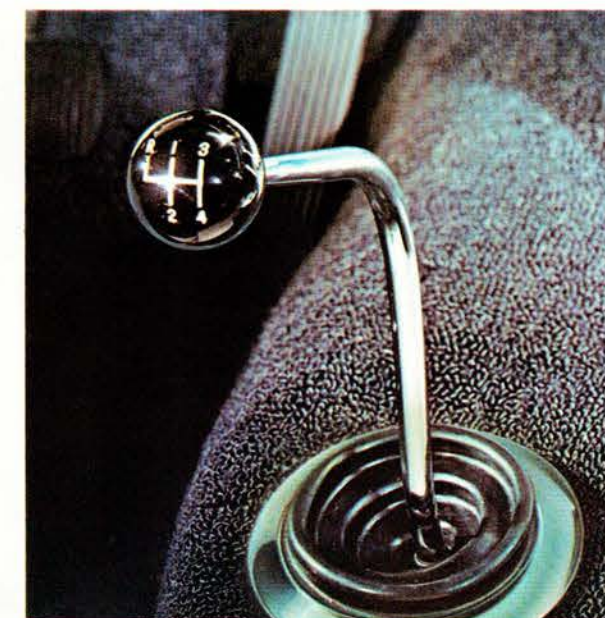
OPTIONAL 4-SPEED TRANSMISSION is a natural for the high-performance, stick-shift fans. All forward speeds fully synchronized.
