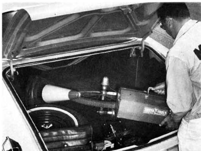
Trunk lip is high enough to make loading and unloading a chore. Spare tire location cuts down usable area, but there's still enough left for the average family.
