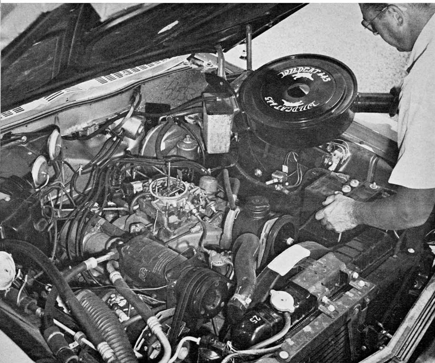
WILDCAT'S ENGINE IS NOT NEW, BUT THE RELIABLE 401-CUBIC-INCH 325-HP POWERPLANT ALREADY OFFERED IN THE INVICTA AND ELECTRA.
