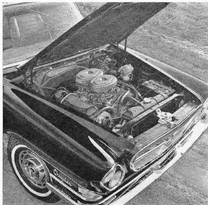
DRY AIR cleaners cover dual 4-throat carburetors.
