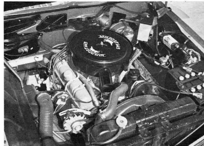
401 CU. IN. ENGINE IS 4 IN. FARTHER FORWARD.
