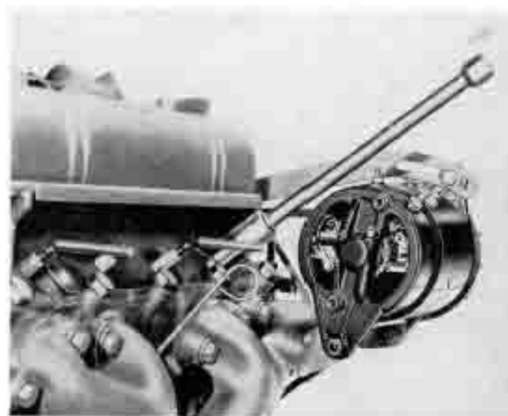
Fig. 18 - Spark-plug removal clearance with generator
