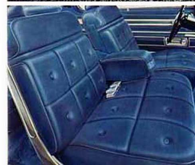
For individualized comfort, you may order a special Brougham interior with this divided (60/40) front seat. Each side has its own seat controls.
