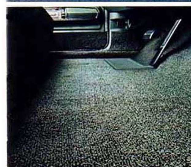
One of the fringe benefits of front drive: a front floor that is completely flat. A middle passenger has no hump in the floor to contend with.
