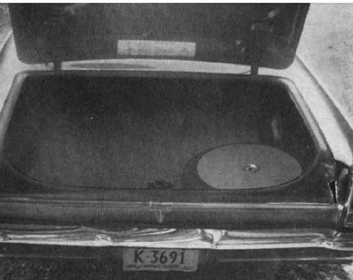
Spare-wheel location is a disappointment, in that it encroaches upon trunk space.
